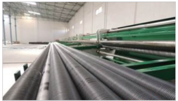
MC ELROY FIN TUBE MACHINE (L, LL & G FIN)
