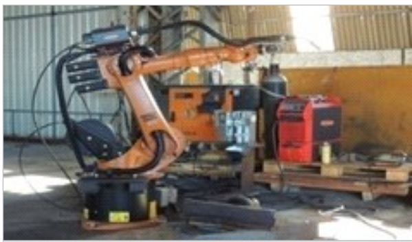
ROBOTIC WELDING MACHINE
