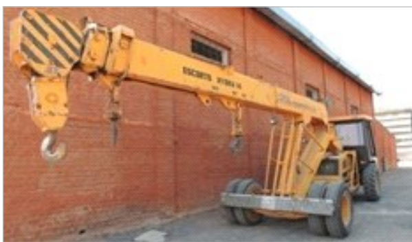
MOBILE HYDRA CRANE
